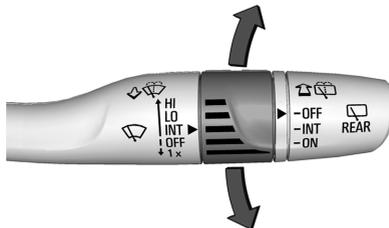
**INT** : Move the windshield wiper lever toward you to spray windshield washer fluid and activate the windshield wipers. The wipers will continue until the lever is released or the maximum wash time is reached. When the windshield wiper lever is released, additional wipes may occur depending on how long the windshield washer had been activated. See *Washer Fluid* ⇨ 250 for information on filling the windshield washer fluid reservoir.
