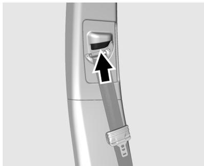
Press and hold the release button while raising or lowering the height adjuster to the desired position.
