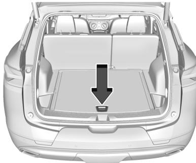
There is storage in the floor of the rear cargo area. Lift the handle to access the cargo management system.
