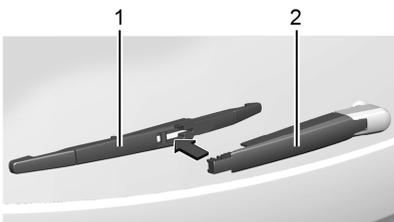
3. Align the new wiper blade assembly (1) with the wiper arm (2) and install by pushing up on the wiper blade assembly until it clicks into place on the wiper arm.
