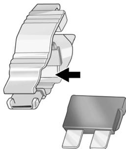
3. Use the fuse puller to remove the fuse from the top or side.
