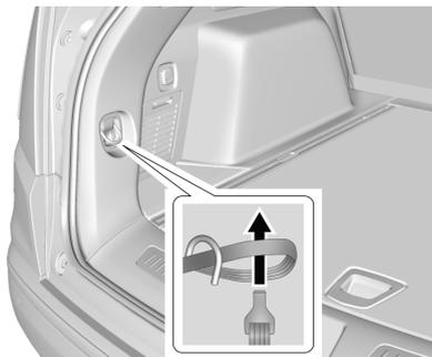
4. Place the loop end of the strap through the cargo tie-down. Place the hook end of the strap through the loop and pull it until the strap is fastened securely to the tie-down.
