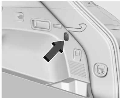
There is a shopping bag hook on each side of the rear cargo area. Press the hook to open. The maximum weight per hook is 5 kg (11 lb).
