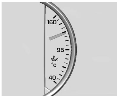
This gauge shows the engine oil temperature.
