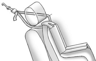
If the position you are using has an adjustable headrest or head restraint, adjust it accordingly to allow proper fitment. If you are using a dual tether, route the tether around the headrest or head restraint posts.
