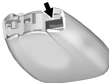
2. Separate the two halves of the remote key using a flat tool inserted into the area near the key slot.
