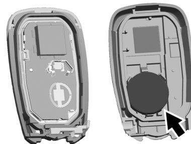
3. Remove the battery by pushing on the battery and sliding it toward the bottom of the remote key. Do not use a metal object.
