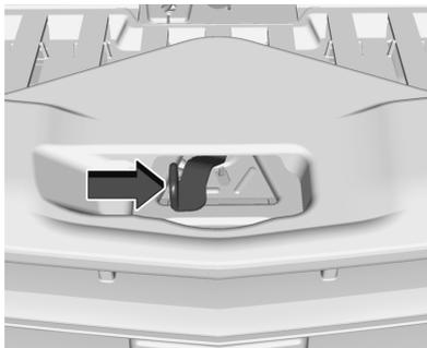
2. Go to the front of the vehicle and locate the secondary release lever under the front center of the hood. Push the secondary hood release lever to the right to release.
