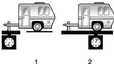
The trailer tongue weight (1) should be 10–15% of the loaded trailer weight (2). Some specific trailer types, such as boat trailers, fall outside of this range. Always refer to the trailer owner's manual for the recommended trailer tongue weight for each trailer. Never exceed the maximum loads for your vehicle, hitch and trailer.
