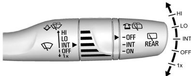
With the ignition on or in ACC/ACCESSORY, move the windshield wiper lever to select the wiper speed.
