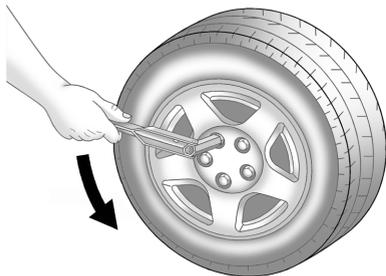
2. Turn the wheel wrench counterclockwise to loosen all the wheel nuts, but do not remove them yet.
