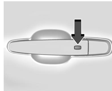
The remote key must be within 1 m (3 ft) of the liftgate or door being opened. Press the button on the door handle to unlock. See “Keyless Access Operation” in *Remote Key Operation* ⇨ 7.
