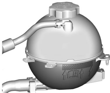
Check to see if coolant is visible in the coolant surge tank. If the coolant inside the coolant surge tank is boiling, do not do anything else until it cools down. See *Engine Overheating* ⇨ 249.
