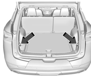
Two cargo tie-downs are located in the rear compartment of the vehicle. The tie-downs can be used to secure small loads.
