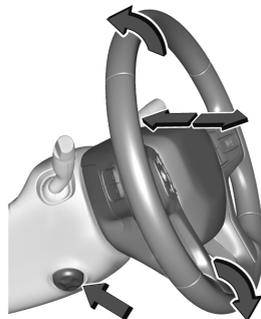
If equipped, the control is on the left side of the steering column.
