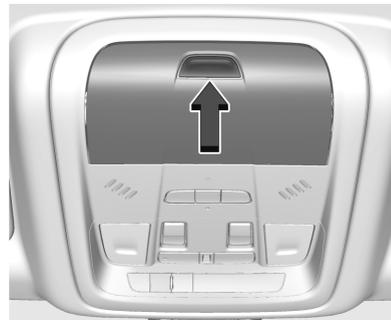
If equipped, sunglasses storage is on the overhead console. Press the fixed button on the cover and release to access.
