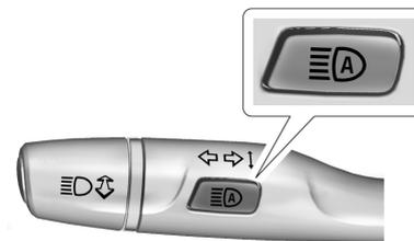
To enable the IntelliBeam system, press **≡A** on the turn signal lever when it is dark outside and the exterior lamp control is in AUTO or **☀**.
