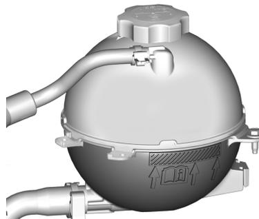
3. Fill the coolant surge tank with the proper mixture to the indicated level mark.
