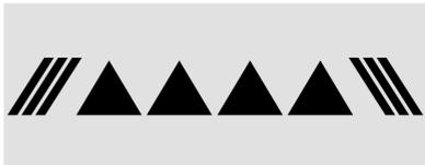
When your vehicle approaches another detected vehicle too rapidly, the red FCA display will flash on the windshield. Also, eight rapid high-pitched beeps will sound from the front, or both sides of the Safety Alert Seat will pulse five times. When this Collision Alert occurs, the brake system may prepare for driver braking to occur more rapidly which can cause a brief, mild deceleration. Continue to apply the brake pedal as needed.
