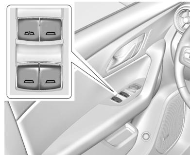
The power windows work when the ignition is on, in ACC/ACCESSORY, or when Retained Accessory Power (RAP) is active. See *Retained Accessory Power (RAP)* ⇨ 187.
