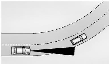
When following a vehicle and entering a curve, ACC may not detect the vehicle ahead and may accelerate to the set speed. When this happens, the vehicle ahead indicator will not appear.
