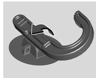
1. Insert one side of the load floor hook into the holder.
