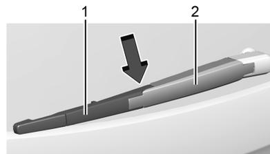
2. While holding the wiper arm, press down at the end of the wiper blade assembly (1) where it attaches to the wiper arm (2) to remove the wiper blade assembly from the wiper arm.
