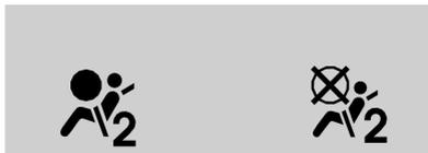
When the vehicle is started, the passenger airbag status indicator will light the symbols for on and off for several seconds as a system check. Then, after several more seconds, the status indicator will light the on or off symbol to let you know the status of the front outboard passenger frontal airbag.
