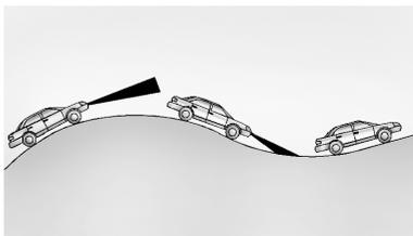
Do not use ACC when driving on steep hills or when towing a trailer. ACC will not detect a vehicle in the lane while driving on steep hills. The driver will often need to take over acceleration and braking on steep hills, especially when towing a trailer. If the brakes are applied, the ACC disengages.
