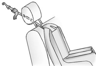
If the position you are using has an adjustable headrest or head restraint, adjust it accordingly to allow proper fitment. If you are using a single tether, route the tether in between the headrest or head restraint posts.
