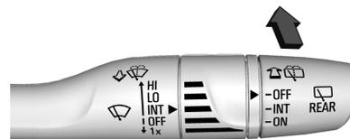
If equipped, push the windshield wiper lever forward to spray washer fluid on the rear camera lens. The lever returns to its starting position when released. See *Rear Camera Mirror* ⇨ 25.
