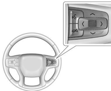
**< or >** : Press to move left or right between the interactive display zones in the cluster. Press the thumbwheel to select.
