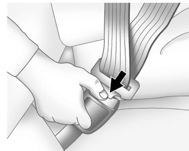
To unlatch the belt, push the release pushbutton on the buckle. The belt should return to its stowed position.
