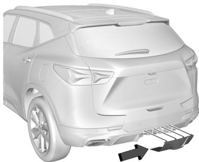
To remove the hitch cover, if equipped:
