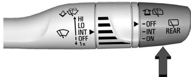
The rear window wiper/washer controls are on the end of the windshield wiper lever.
