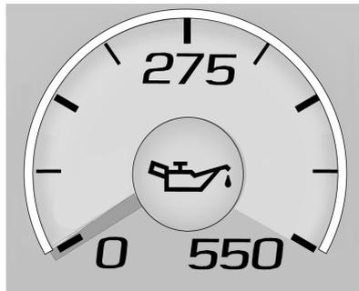
The engine oil pressure gauge shows the engine oil pressure in kPa (kilopascals) when the engine is running.
