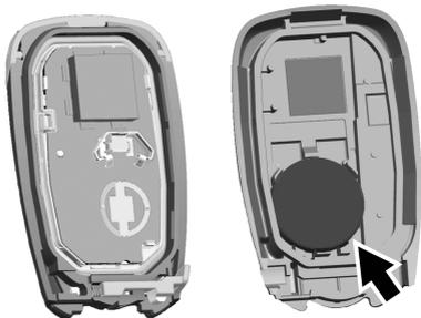
3. Remove the battery by pushing on the battery and sliding it toward the bottom of the remote key.
