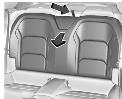
Pull the loop on the center of the rear seat back. The rear seat back will fold down.
