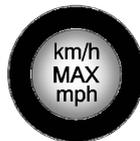
20. If the flat tire was able to inflate to the recommended inflation pressure, remove the maximum speed label from the sealant canister and place it in a highly visible location.
