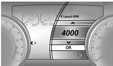
8. Adjust the desired RPM using  $\triangle$  or  $\nabla$ : 1800–4000 RPM for manual transmissions and 1200–2400 for automatic.
