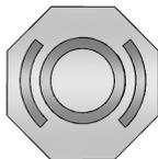
The brake/clutch master cylinder reservoir is filled with GM approved DOT 4 brake fluid as indicated on the reservoir cap. See *Engine Compartment Overview* ⇨ 222 for the location of the reservoir.
