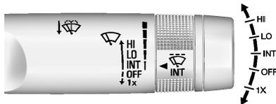
The windshield wiper/washer lever is on the right side of the steering column. With the ignition on or in accessory mode, move the windshield wiper lever to select the wiper speed.
