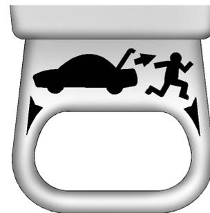
There is a glow-in-the-dark emergency trunk release handle on the trunk lid. This handle will glow following exposure to light. Pull the release handle to open the trunk from the inside.
