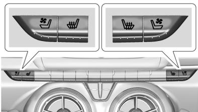
If available, the engine must be running to operate.
