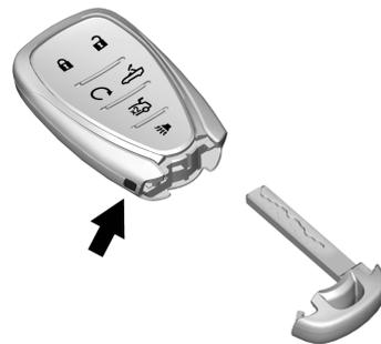
1. Press the button on the side of the remote key and pull the key out. Never pull the key out without pressing the button.
