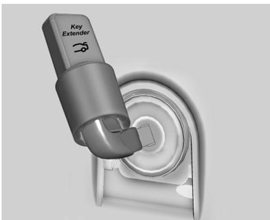
6. Place the key extender over the key head until the key extender stops.
