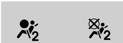
The symbol for on and off will be visible during the system check. When the system check is complete, either the symbol for on or off will be visible. See *Passenger Airbag Status Indicator* ⇨ 89.
