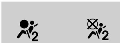
The symbols for on and off will be visible during the system check. When the system check is complete, either the symbol for on or off will be visible. See *Passenger Airbag Status Indicator* ⇨ 87.
