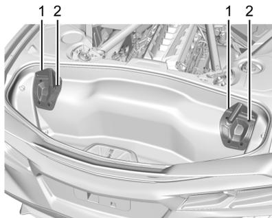
2. Remove the four lift off bracket bolts (2) to remove the brackets (1).
