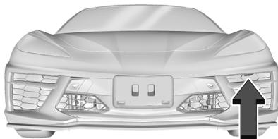
1. Locate the touchpad in the grill opening near the driver side headlamp.
