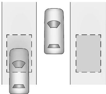
The SBZA sensor covers a zone approximately one lane over from both sides of the vehicle, or approximately 3.5 m (11 ft). The height of the zone is approximately between 0.5 m (1.5 ft) and 2 m (6 ft) off the ground. This zone starts at approximately the middle of the vehicle and goes back 5 m (16 ft).
