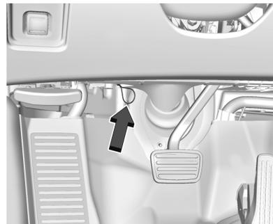
1. Locate the manual release cable loop to the left of the brake pedal.
