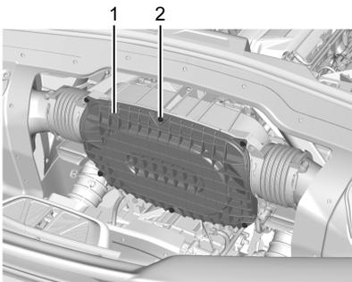
6. Remove the air cleaner cover screws (2) and cover (1).
