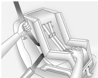
7. To tighten the belt, push down on the child restraint, pull the shoulder portion of the belt to tighten the lap portion of the belt, and feed the shoulder belt back into the retractor.
