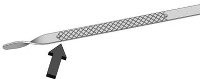
If the oil is below the cross-hatched area at the tip of the dipstick, add 1 L (1 qt) of the recommended oil through the oil fill cap opening in the oil tank fill tube and then recheck the level. See “Selecting the Right Engine Oil” later in this section for the type
