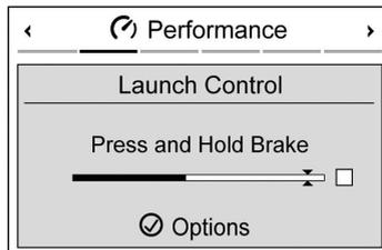
1. Using the DIC buttons on the right side of the steering wheel, navigate to the performance menu. See *Instrument Cluster* ⇨ 79.
