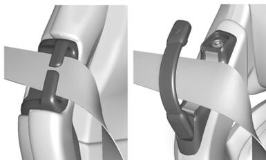
2. Be sure that the shoulder belt is routed through the seat belt guide. See *Lap-Shoulder Belt* ⇨ 47 for proper belt routing.
