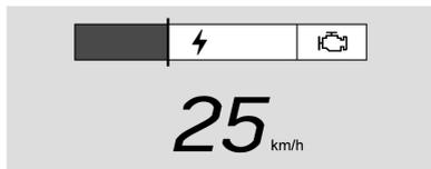
**Stealth** : Displays the vehicle speed and the battery capability gauge. This includes the battery propulsion capability of the vehicle. Stealth view is only available in Stealth Mode. See *Driver Mode Control* ⇨ 187.
