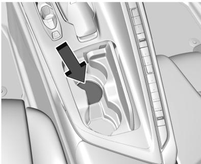
1. Place the remote key in the front cupholder with the mechanical key end facing up.
