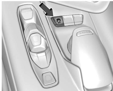
The TCS/StabiliTrak/ESC button is on the center console.
