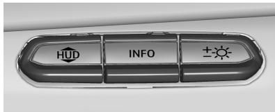
The HUD control is to the right of the steering wheel on the instrument panel.
