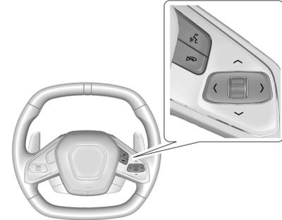
Press < or > to access the cluster applications. Use the thumbwheel to scroll ^ or v through the list of available features. Press the thumbwheel to select. Not all applications will be available on all vehicles.
