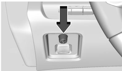
This feature adjusts the brightness of all illuminated controls. The knob for this feature is on the left side of the instrument panel.
