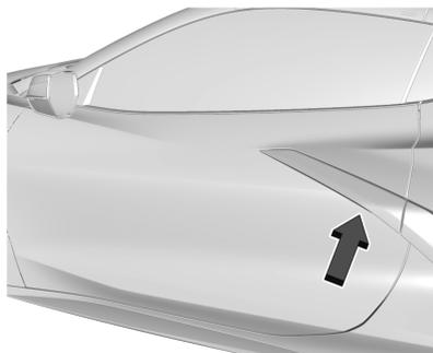
For Keyless Access, hold the remote key within 1 m (3 ft) of the door handle. Grip and press the door handle touchpad. See *Remote Key Operation* ⇨ 7. This feature can be programmed. To view available settings from the infotainment screen, touch Settings > Vehicle > Remote Lock, Unlock, Start.
