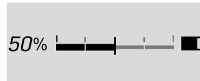
This displays the high voltage battery state of charge, and is shown in the Shuttle and Stealth mode. The value at the left is an estimate of how much high voltage battery state of charge remains.
