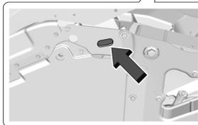
Use only a service jack with a lifting pad diameter of 64 mm (2.5 in) or smaller, and thick enough to make sure the jack does not contact the vehicle body.
