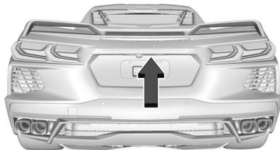
Press the hatch/trunk release touchpad to open the trunk if the remote key is within 1 m (3 ft).
