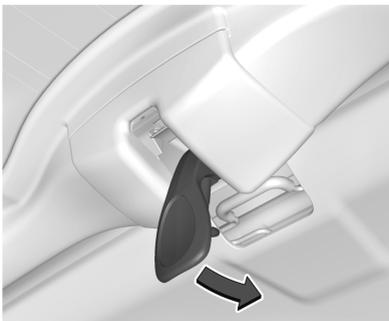
10. Push back and up on the rear release handle to insert the hook in the loop.
