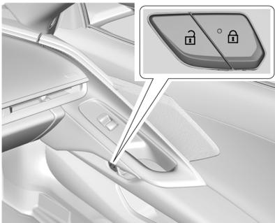
The passenger power door lock switch can also be used to lock or unlock the doors. The fuel door, hood, and hatch/trunk are also locked and unlocked using either power door lock switch.
