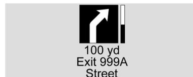
**Navigation** : If equipped, displays turn-by-turn navigation information when navigation is active and an upcoming maneuver is pending. It appears until the maneuver is complete, then the HUD image returns to the previous view.
