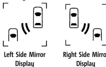
When the vehicle is started, both outside mirror SBZA displays will briefly come on to indicate the system is operating. When the vehicle is in a forward gear, the left- or right-side mirror display will light up if a moving vehicle is detected in that blind zone. If the turn signal is activated in the same direction as a detected vehicle, this display will flash as an extra warning not to change lanes.
