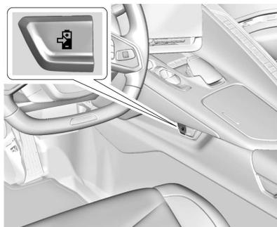
Press the Charge+ button on the drive side of the center console. When the Charge+ feature is active, the hybrid battery charging light displays on the DIC. See *Hybrid Battery Charging Light* ⇨ 84. Also, a small pop-up window will also appear showing the exact SOC and electric power input/output. The
