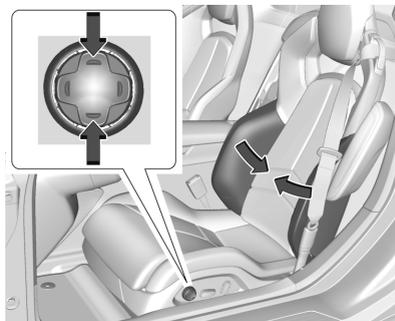
If equipped, press and hold the control upward to increase or downward to decrease the side bolster support.
