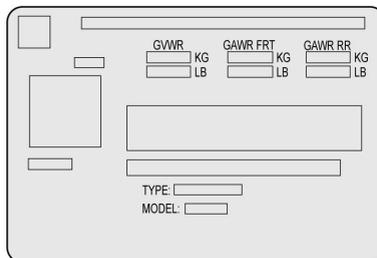
A vehicle-specific Certification label is attached to either the rear edge of the driver door or the B-pillar. It may show the gross weight capacity of the vehicle, called the Gross Vehicle Weight Rating (GVWR). The GVWR includes the weight of the vehicle, all occupants, fuel and cargo.
