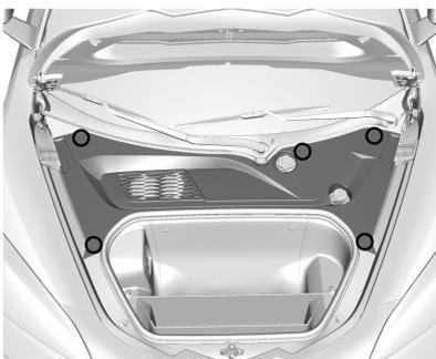
6. Release the five clips and remove the outer cover to access the battery.
