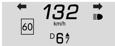
**Tour** : Displays the vehicle speed, gear position, shift indicator, and speed sign.
