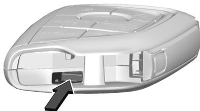
2. Use the mechanical key blade in the slot to remove the battery cover by hand.
