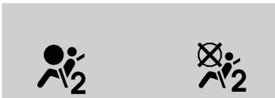
When the vehicle is started, the passenger airbag status indicator will light the symbols for on and off for several seconds as a system check. Then, after several more seconds, the status indicator will light either the on or off symbol to let you know the status of the front outboard passenger frontal airbag.
