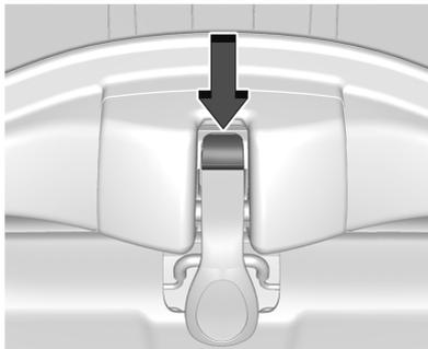
7. Press the button on the front of the rear release handle to unlock it. The latch lever will open.
