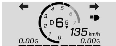
**Sport** : Displays the vehicle speed, a circular tachometer, gear position, shift indicator, and G-Force meter.
