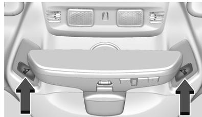
If equipped, the reading lamps are in the overhead console. The lamps go on when any door is opened,
