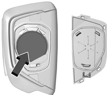
3. Remove the seal by pulling on the tab to access the battery.
