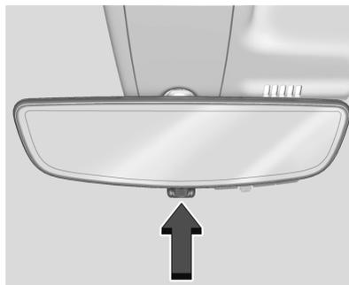
Pull the tab to turn on the display. Push the tab to turn it off. When the display is off, the automatic dimming function is active.
