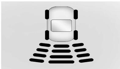
The instrument cluster may have a Park Assist display with bars that show “distance to object” and object location information for RPA. As the object gets closer, more bars light up and the bars change color from yellow to amber to red.
