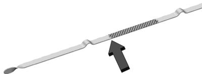
If the oil is below the cross-hatched area at the tip of the dipstick, add 1 L (1 qt) of the recommended oil through the oil fill cap opening in the oil tank fill tube and then recheck the level. See “Selecting the Right Engine Oil” later in this section for the type of oil to use. For engine oil crankcase capacity, see *Capacities and Specifications* ⇨ 313.
