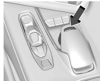
To activate My mode, Weather, Tour, Sport and Track mode, turn the DMC knob on the center console to make a mode selection. When a mode is selected, an indicator will
