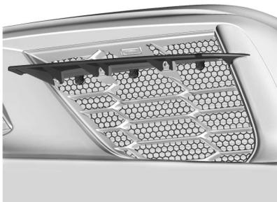
For vehicles with the optional Grille Screen Guards (VWE), remove them for track events when the ambient temperature reaches 32° C (90° F) or higher. See your dealer for complete procedure.
